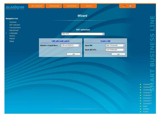
First choose the configuration of the system. If the system is equipped with LNB and multiswitch, so you can select the number of feeds on the left. If the system is operated with a Quattro LNB, so you choose from the right side, which satellite level contact with the corresponding input jack. Press the "OK" button, the corresponding data are loaded and you will be forwarded to the selection of the programs.
