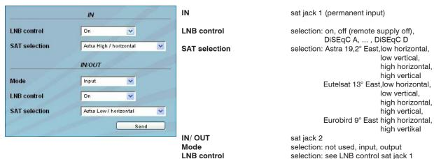
If the 2nd sat jack is configured as a loop-through output, or not used, the associated input configuration parameters "LNB control" and "SAT selection" are grayed out and not adjustable.
