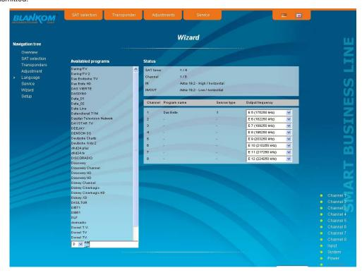
In this way, up to 8 programs per PALIOS module can be selected now to be transferred. First, as the output channel the next higher channel to the last selected program package is offered. But for each program the output channel can be chosen freely in the total frequency range. If an incorrect selection is made, it can be removed by double-clicking the unwanted selected program in the right field.
