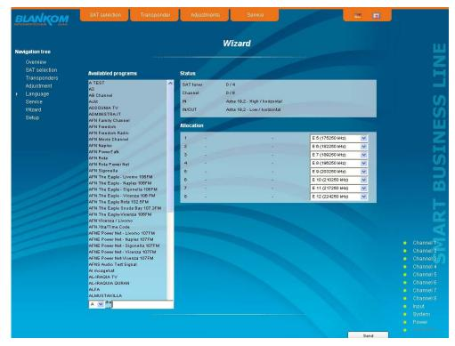
In the left column, all available programs are loaded according to the selected satellite from the database. The listing is in alphabetical order, the start of the list can be selected under the list by selecting the first letter. Alternatively, you can also enter a string (e.g. "HD") in the text box next to the letter sequence. In this case all the programs are listed that contain that search string in their names.
