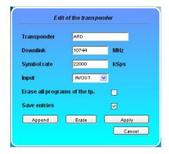
Existing entries can be changed or new ones are attached. By clicking on the appropriate box the program list of the transponder can be deleted and changes or additions can be stored into the database permanently. If the box "Save entries" is not clicked, the changes will remain only as long as the user interface is open. With the next start of the user interface the changes are lost. In this simple way, the program data is kept up to date.
