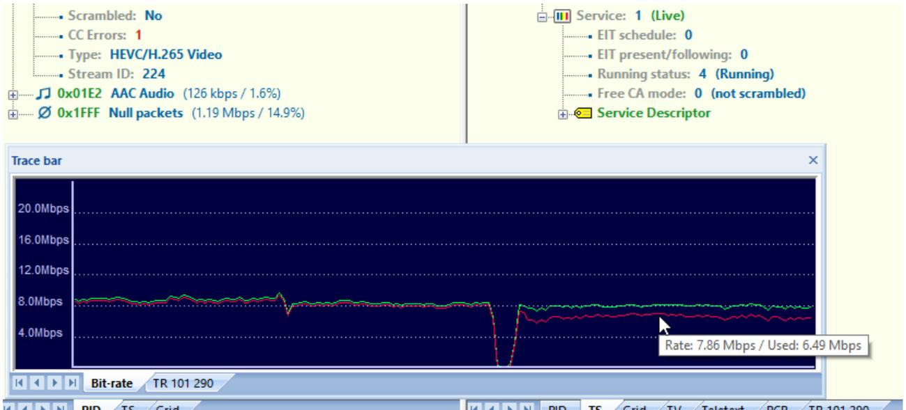
As you can see from the Trace, the former configured max data rate of 8Mb/s encoding is more constant than before and the Video encoder is now more smooth and less data rate.
