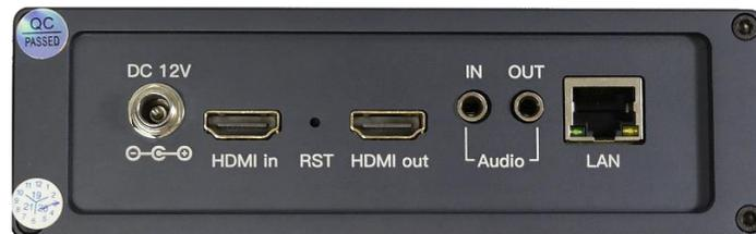
Rear panel: 12V DC Jack ( + = middle), RST=Reset hole, HDMI-Input connector, External Audio-Stereo IN by 3.5mm Jack (not included with the device), Gigabit Ethernet
