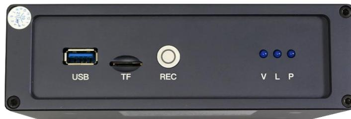
Front-Panel: USB connector for Recording, TF-Card (µ-SDCard), REC-Button, Status LEDs: Power, Ethernet, System ready
