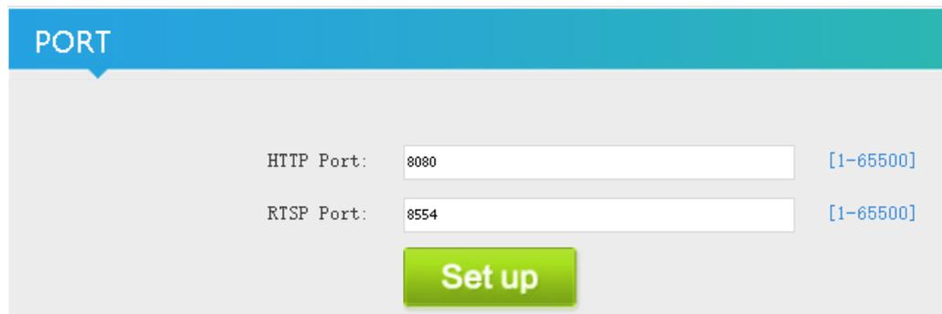
These are the basic ports for HTTP and RTSP-Streaming use. You can modify that but we recommend to keep them as they are because RTSP – receivers might be fixed to that port while HTTP isn't. The bottom of every of the menu-pages contains the 'Set up' buttons to take and enable your changes.
