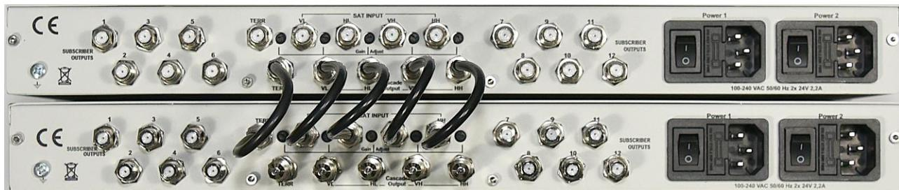
Please take attention to the last BMS in the cascade (or if it will be used w/o cascading but standalone): The 5 terminating resistors with DC-Blockers.
