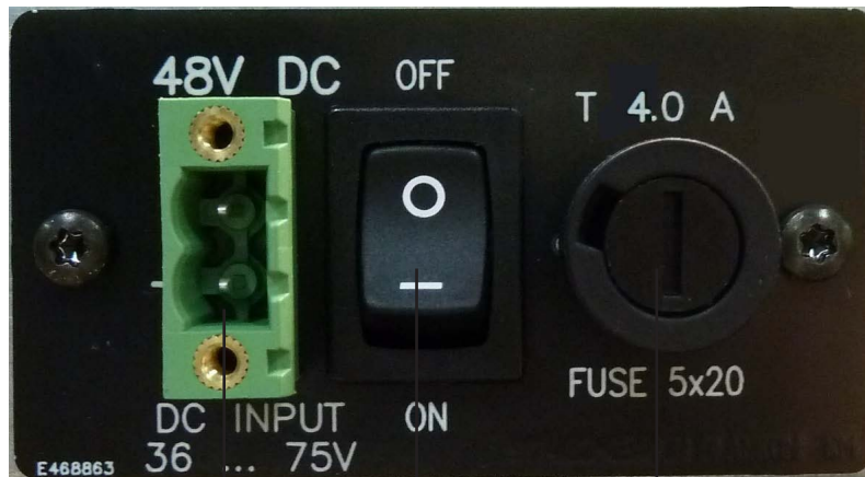
DC connection On/ off switch Fuse
