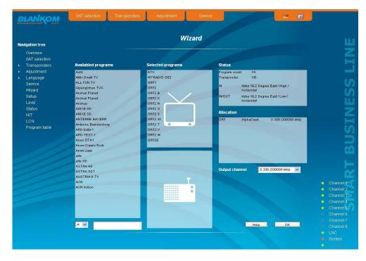
In this way, up to 8 transponders per QAMOS module can be selected now to be transferred. First, as the output channel the next higher channel to the last selected program package is offered. But for each packet the output channel can be chosen freely in the total frequency range. If an incorrect selection is made, it can be removed by double-clicking the unwanted selected transponder in the right field.
