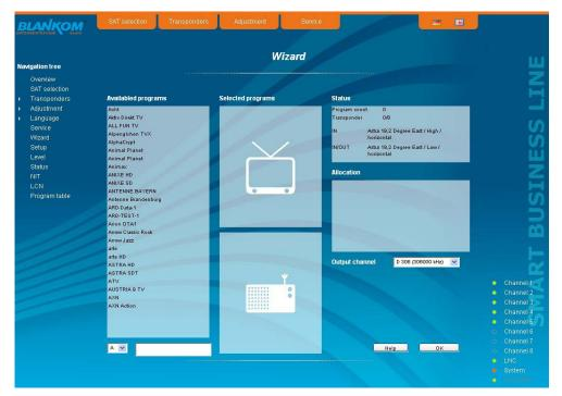
In the left column, all available channels are loaded according to the selected satellite from the database. The listing is in alphabetical order, the start of the list can be selected under the list by selecting the first letter. Alternatively, you can also enter a string (e.g. "HD") in the text box next to the letter sequence. In this case all the channels are listed that contain that search string in their names.
