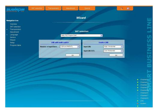
First choose the configuration of the system. If the system is equipped with LNB and multiswitch, so you can select the number of feeds on the left. If the system is operated with a Quattro LNB, so you choose from the right side, which satellite level contact with the corresponding input jack. Press the "OK" button, the corresponding data are loaded and you will be forwarded to the selection of the channel or transponder.
