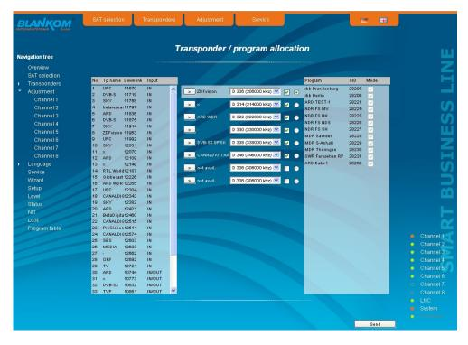
To make changes, you must first select the desired channel. This is done either by clicking the appropriate selector outside right next to the output channel in the middle of the channel list or by clicking on "Channel" in the navigation tree on the left side, which is listed as a point of the menu "Transponders".
