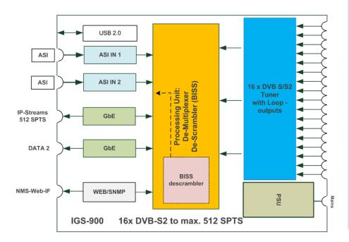
BLANKOM IGS-900 is a DVB/IP Gateway, which has 16 DVB-S/S2x tuners (DVB-C, DVB-T/T2 optional) and de-multiplexing functions in 1RU chassis to convert RF signals into SPTS or MPTS IPTV output.
